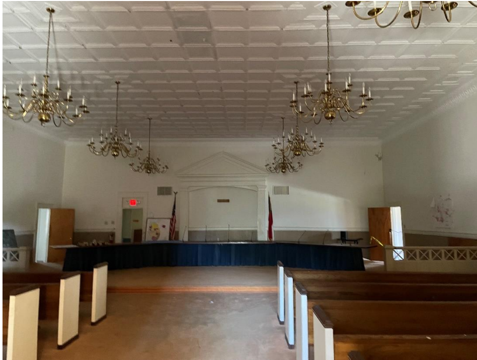
Photo 27 – View of courtroom on the second floor. Assume porous materials are mold impacted (carpet, fabric, benches, etc.).
