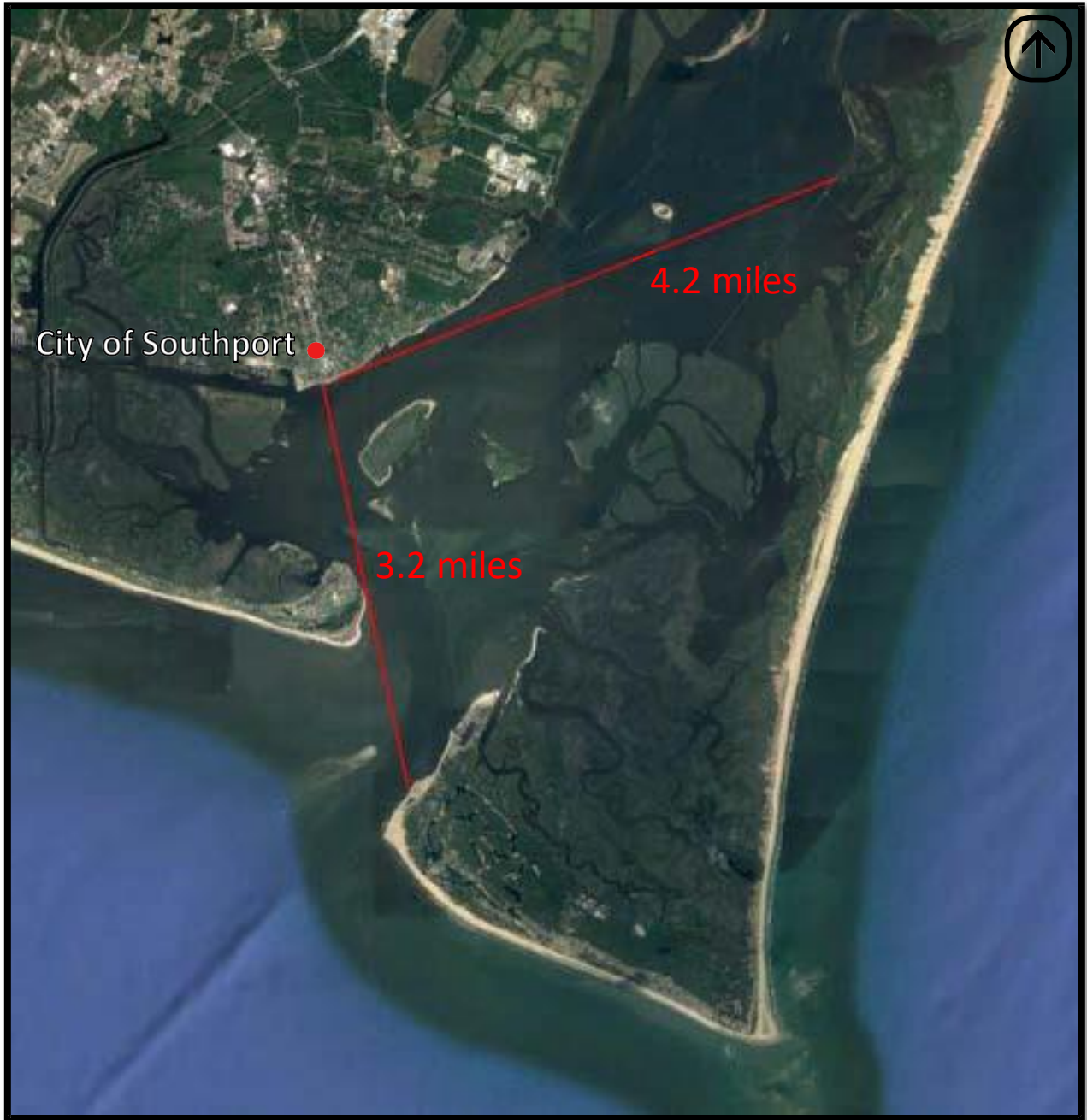
Figure B-1: Location map depicting the location of the Southport shoreline in Brunswick County, NC and the fetch length across different fetch windows.
